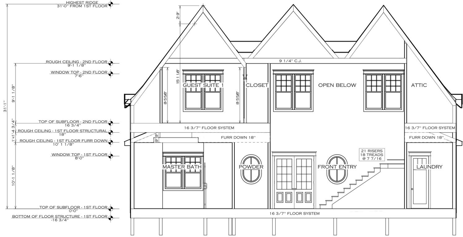
**S1 CROSS SECTION: FRONT ELEVATION**
